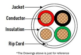
4 Core 18AWG Stranded Copper Conductor Individual insulation of High-Quality FRPVC Outer Sheath PVC cover with anti-flame CM Ratings
